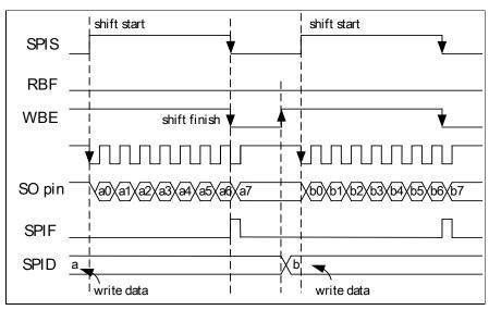
Fig. 5-14 Transmit Mode (8-bit, 1 word)
